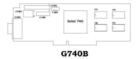
The layouts for the two cards are the same, the different between the G740A and the G740B is that the G740A uses 4MB(or 8MB)of SGRAM, and the G740B used 8MB of SDRAM
